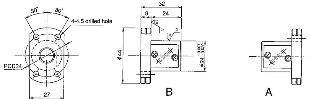
Select the orientation of nut flange by circling A or B.
